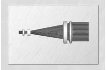
Air-spaced 4-element optics
