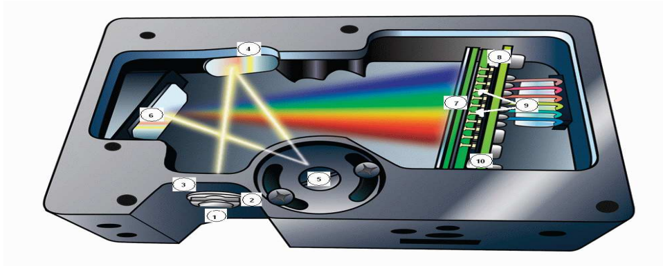
Figure 8: Inside view of the Ocean Optics USB 4000 Spectrometer. 1: connector used to plug the fiber. 2: slit acting like the entrance aperture. 3: absorbance filter, used to block second- and third- order effects or to balance color. 4: collimating mirror. 5: prism. 6: focusing mirror. 7: detector collection lens used to increase light-collection efficiency. 8: filter. 9: quartz window to enhance the performance of the spectrometer. 10: CCD camera
