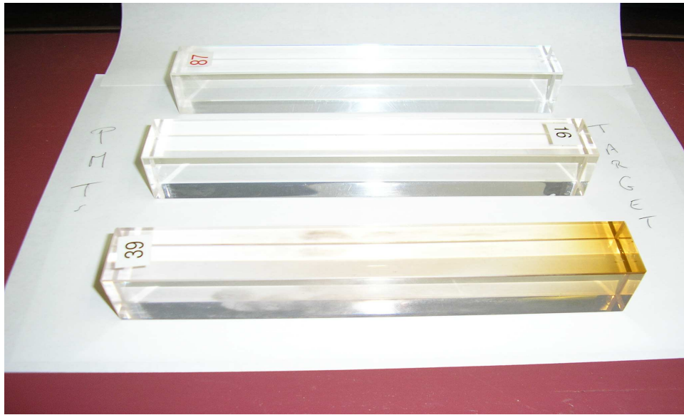
Figure 22: Visual inspection of blocks 39, 87 and 101. The block 16 in this picture is actually the block 101. the surface of block 39 us scratched, and the the PMT side of blocks 39 and 101 are darkened.
