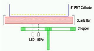
The equipment connected to the photomultiplier tube converts the analog signals of the light intensity produced into more easily read digital signals. The procedure that will be used to measure the scintillation rate involves measuring with AC current. The chopper's purpose is to cut the
