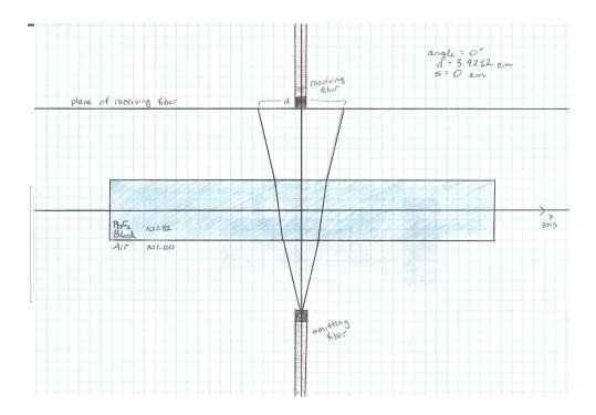
Using the program, we computed d and s with a beginning angle of 2.5 degrees. When the fiber holder is angled so that the incident angles are altered by 2.5 degrees, d is equal to 3.9294 cm. Therefore *d* only has a change of 12 micrometers. With the same angle, *s* is calculated to be only about half of a millimeter.
