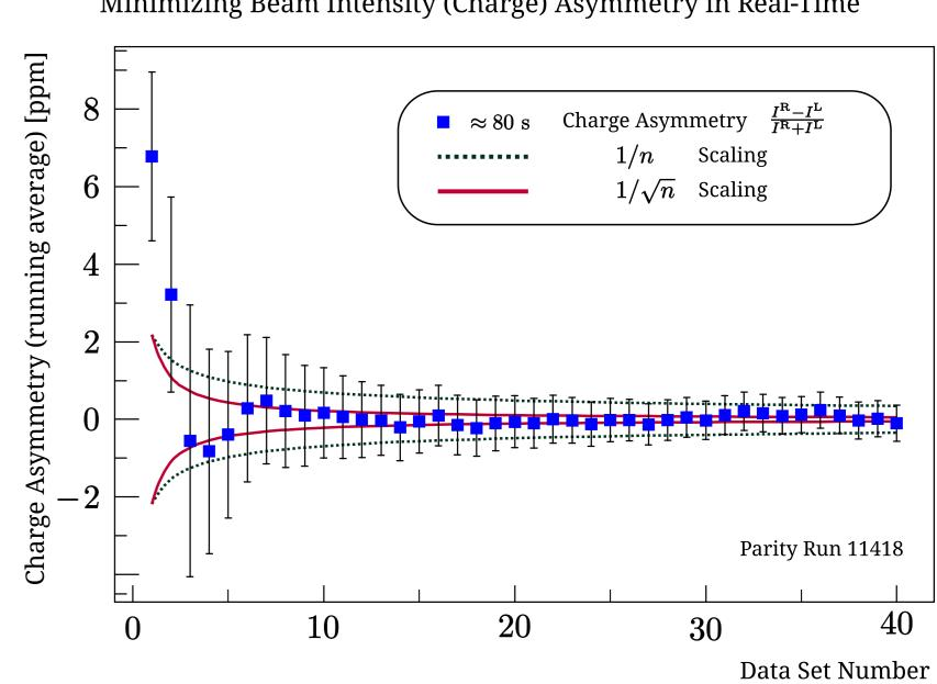
We also monitor and record the beam position differences between two helicity states at the beginning of the beam line (Injector) and at the experimental Hall for Qweak (Hall C). And recorded data are used to extract the position sensitivities to the asymmetry  $A_{LR}^p$ . So far we have achieve the position sensitivities contribution to  $A_{\rm LR}^p$  below 0.2 ppm.
