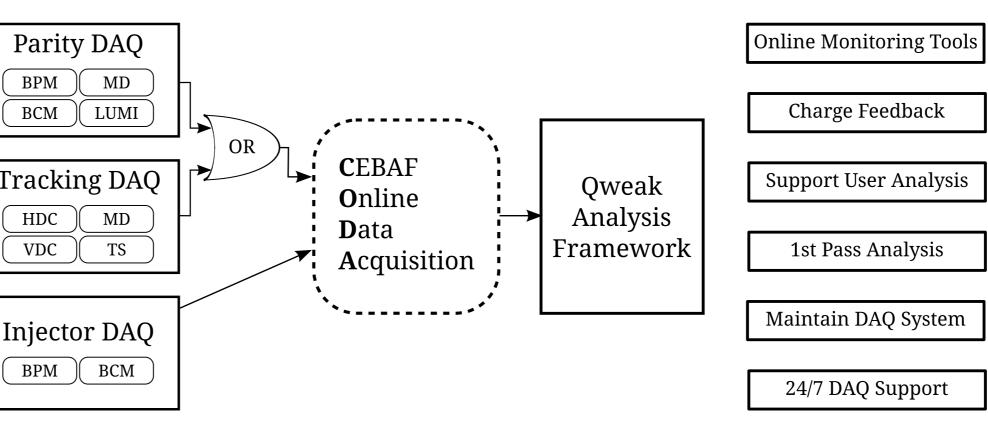
Cherenkov Detector rate 800MHz each, total 6.4GHz in Parity Mode Parity Mode Raw data is about 20GiB/hr or about 480GiB/day • 22 sampling ADCs for Parity DAQ, 12 sampling ADCs for Injector DAQ, 18 TDCs for Tracking DAQ, and others ADCs and scalers.
