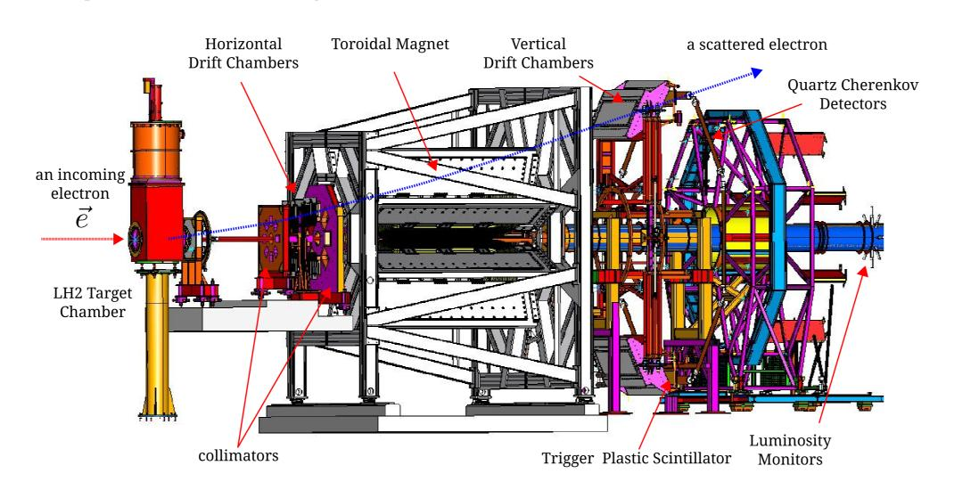
The elastically scattered electrons are focused through collimators and through the toroidal magnet toward Cherenkov detectors. The Cherenkov detectors are arranged symmetrically around the beamline. The current signals of the Cherenkov detectors are converted
