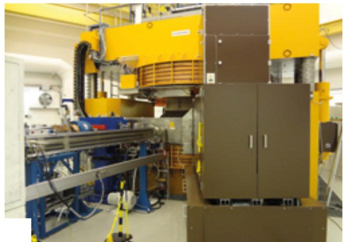
The cyclotron at RADEF in Finland, which is used to test the radiation hardness of electronics to be used in space.
