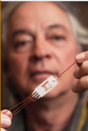
■ Sandia's 'neutristor', which exploits deuterium fusion to generate neutrons. [Credit Sandia National Laboratories].
