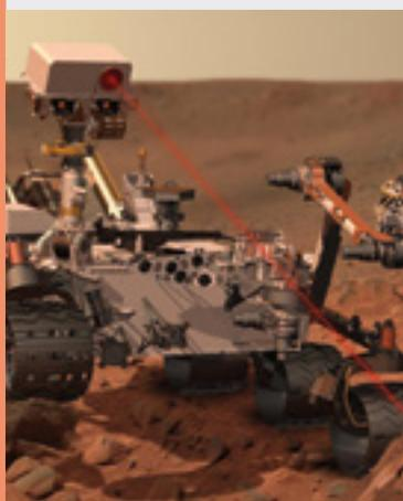
long as an Earth year) there is not enough energy in the light from the Sun. The rover needs the 110 watts from the nuclear power pack to carry out a range of experiments with electrically powered instruments. It should last for about 14 years.
