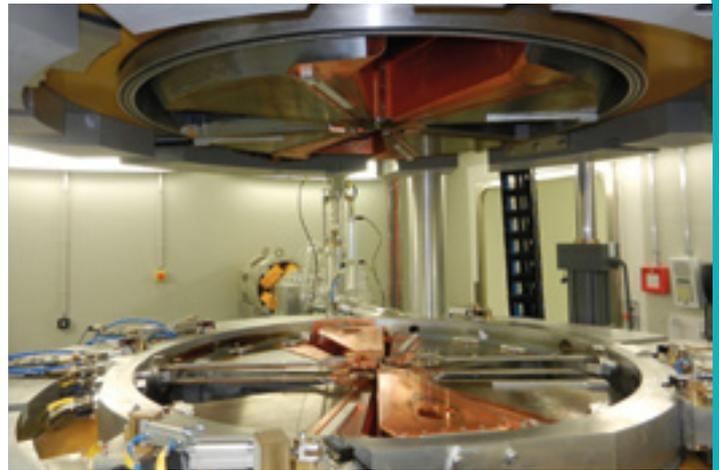
■ Inside the cyclotron used to make medical radioisotopes at the University of Bern Hospital in Switzerland.
