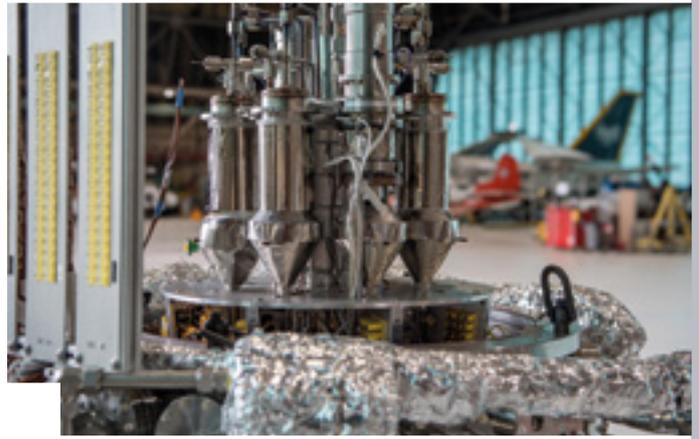
The prototype NASA nuclear reactor, Kilopower, designed for space travel. [Credit NASA].
