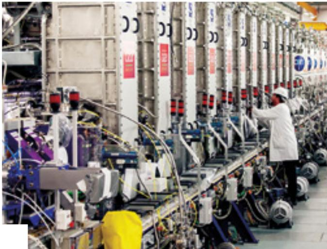
This is part of a new linac, SPIRAL2, at the one of Europe's major nuclear physics facilities, GANIL (Grand Accélérateur National d'Ions Lourds) in Caen, France. The accelerator uses an advanced superconducting accelerating system to create beams of a wide variety nuclei for nuclear physics experiments.
